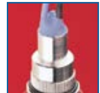
5. Pot cable using liquid or putty
