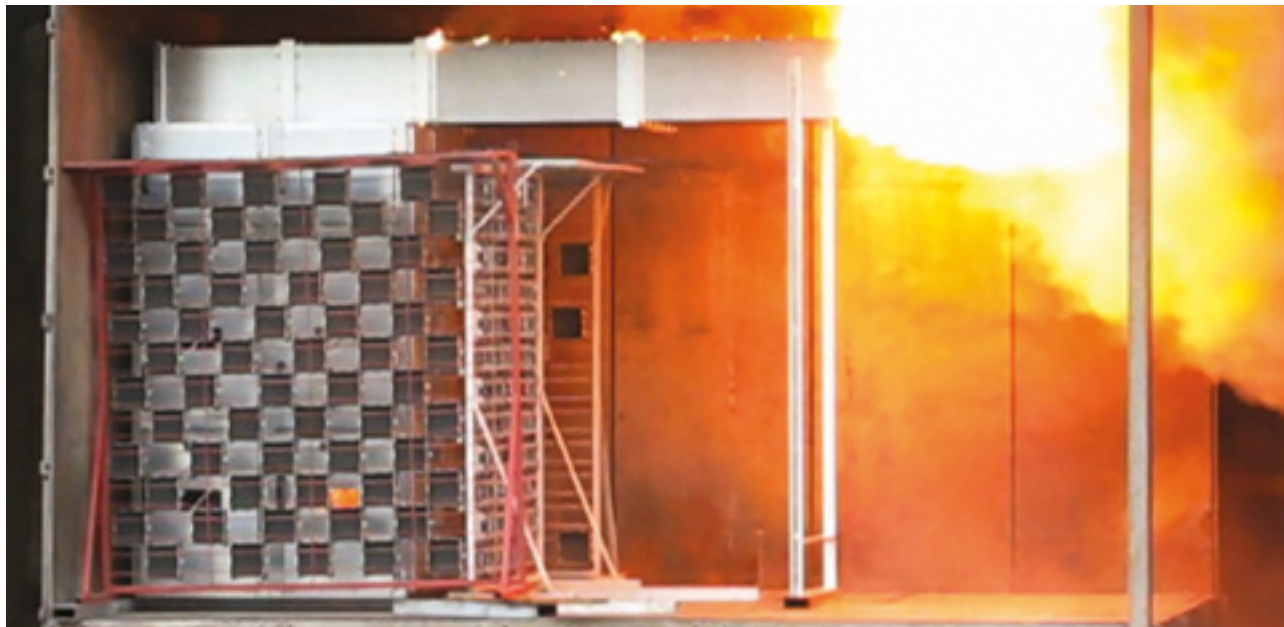
Internal arc fault test, 31.5kA/1s
